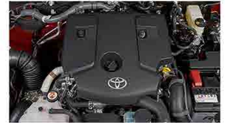
2.8L 1GD ENGINE WITH 201 HP MAX OUTPUT & 500 NM MAX TORQUE
